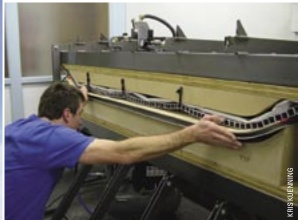
Alex carefully puts the skis in the purpose built pneumatic press.
