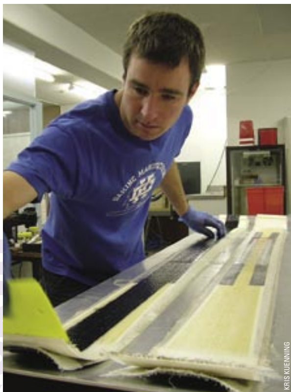
Kingswoods handmade construction of bamboo, fibreglass and carbon fibre.
